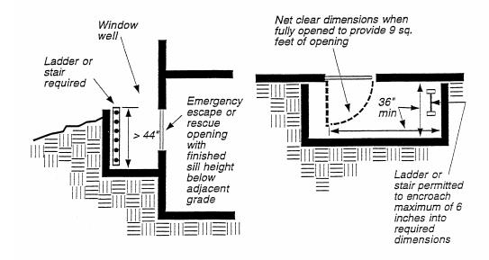
WINDOW WELL is a soil-retaining structure at a window having a sill height lower than the adjacent ground elevation. Section 224
