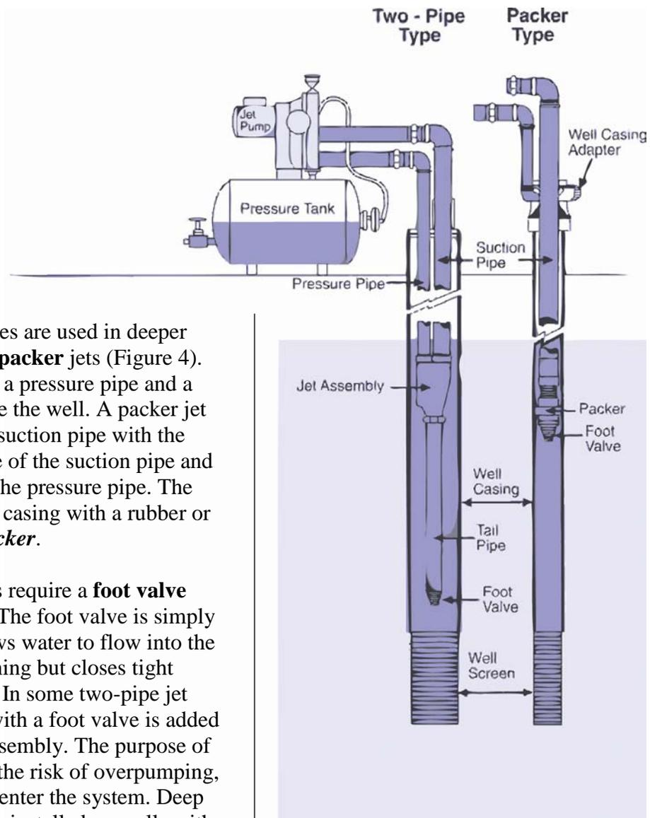
Two types of jet assemblies are used in deeper wells: **two-pipe** jets and **packer** jets (Figure 4). The two-pipe jet has both a pressure pipe and a suction pipe located inside the well. A packer jet uses a single pipe for the suction pipe with the space between the outside of the suction pipe and the well casing acting as the pressure pipe. The inner pipe is sealed to the casing with a rubber or leather gasket called a *packer*.
