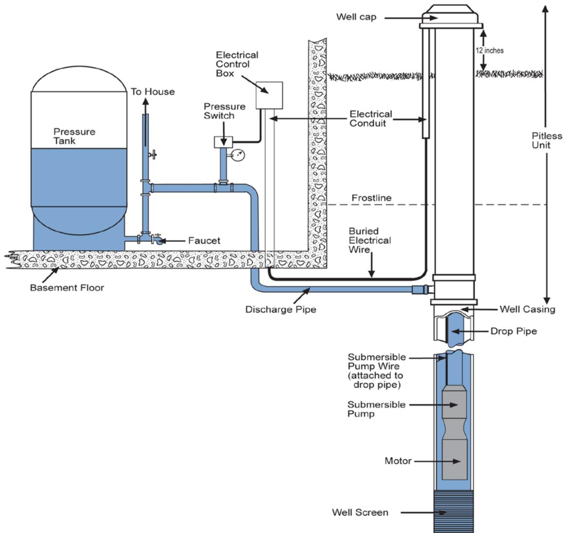
FIGURE 3 Well and Water System.
